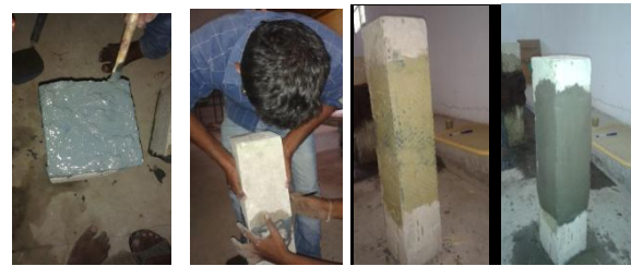
Fig.3 Joining with SBR modified cement paste, Attached Chicken Wire Mesh on Epoxy coating and Plastered with SBR modified cement mortar
