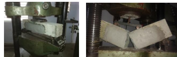
Fig. 4 Testing of Beam Repaired with Epoxy, SBR + Cement Modified Latex and Welded Mesh (RESC- WLM)
